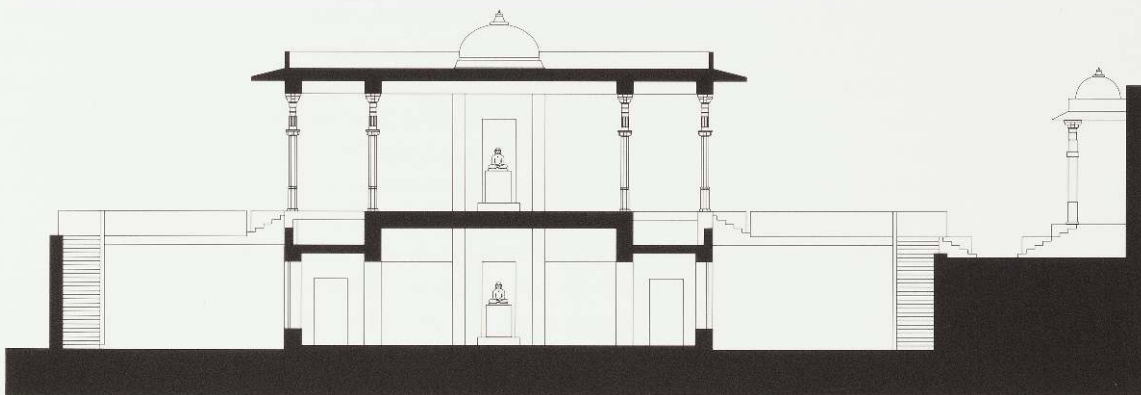
Fig. 53 The two floor levels of the Simandhara Svāmī Temple (above) and the Guru Mandir (below), and a section of the two-storeyed temple at Jalor.
