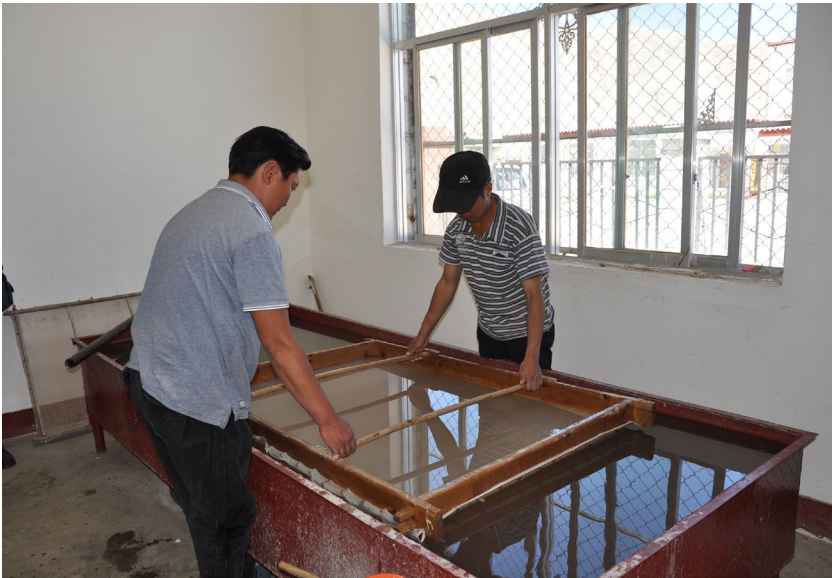
Figures 6.5 and 6.6 The process of making paper in Nyemo, Central Tibet. Process of shaping the sheet of paper. Photograph by the author, 2013.
