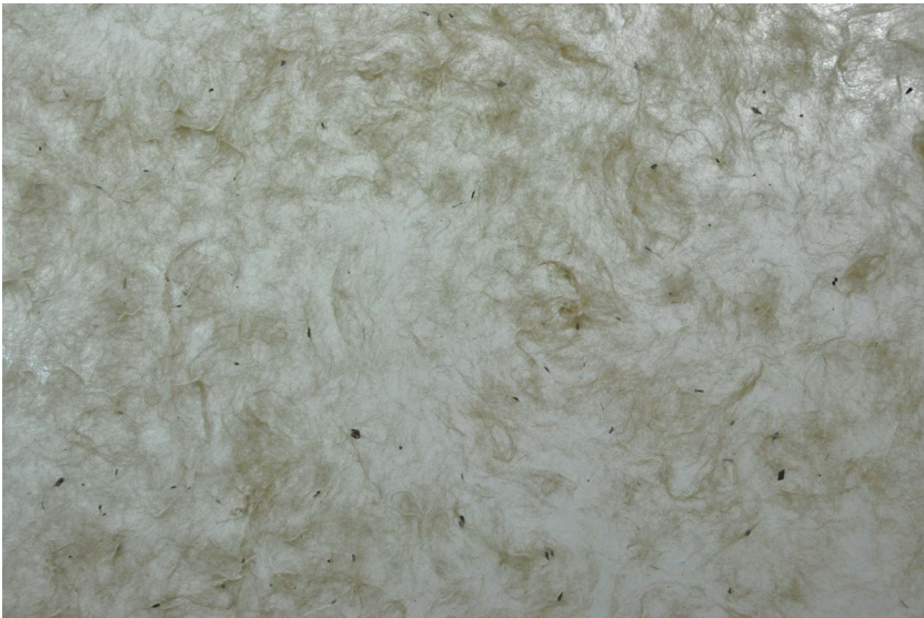
Figure 6.4 A woven type of paper made with a floating mould constructed with a wooden frame and attached woven textile. Photograph by the author, 2016.
