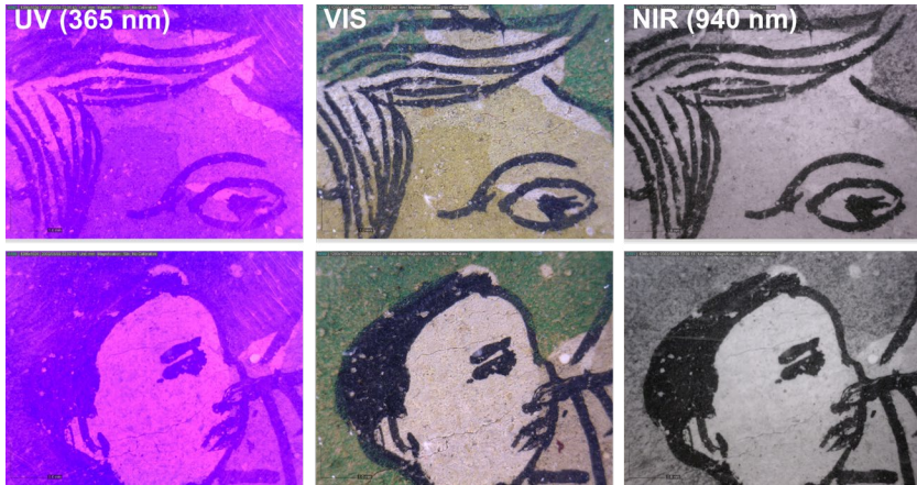
Figure 7.3 Two-wavelength reflectography, carried out with a hand-held USB microscope equipped with in-built light sources at 365 nm (left column) and 940 nm (right column), and an external lamp in the visible range (middle column). While most colourants become transparent in the NIR (near-infrared), carbon ink absorbs significantly in this wavelength range and appears black. The UV image makes corrections—or in this case damage—more obvious.
