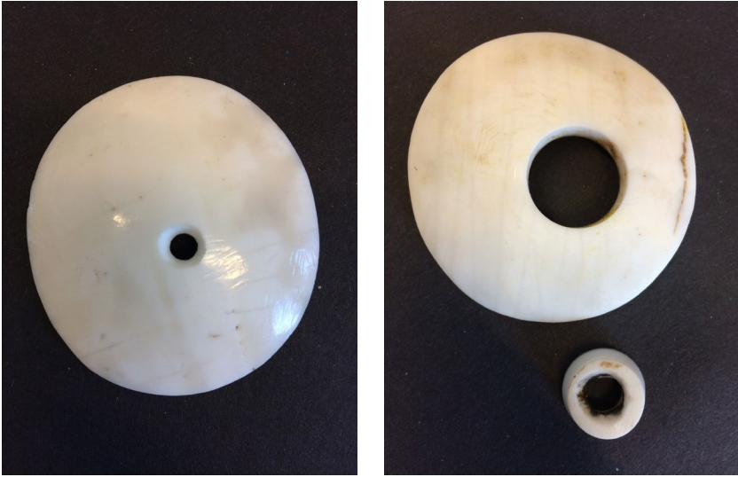
Figures 5.3 and 5.4 Prayer wheel washers. The washer in Figure 5.3 is new. The washer in Figure 5.4 has been worn down and split in two by the bamboo tube that rotates on top of it.
