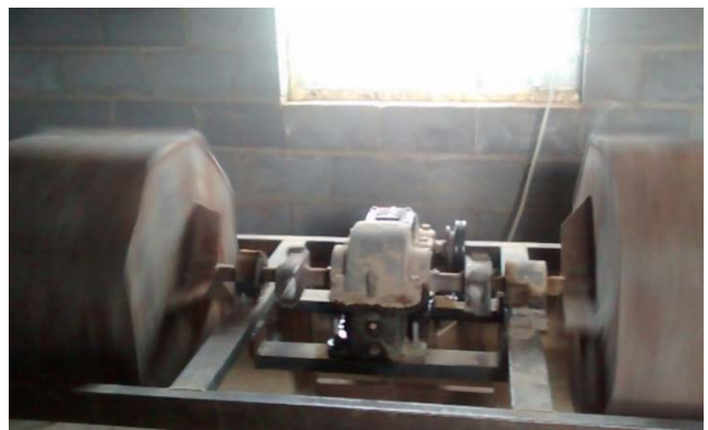
Fig. 2: Self-built rotating machines which are filled with iron balls and stones which over several hours are grinded into sands.
