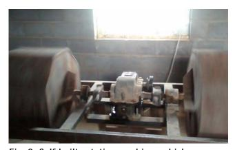
Fig. 2: Self-built rotating machines which are filled with iron balls and stones which over several hours are grinded into sands.
