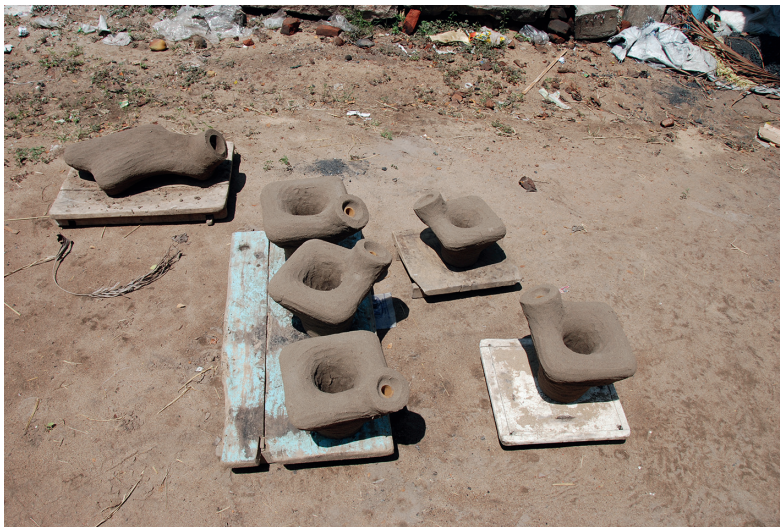
Fig. 7. Clay moulds, Swamimalai bronze casting workshop, February 2014. Photo: Anna A. Ślącza
