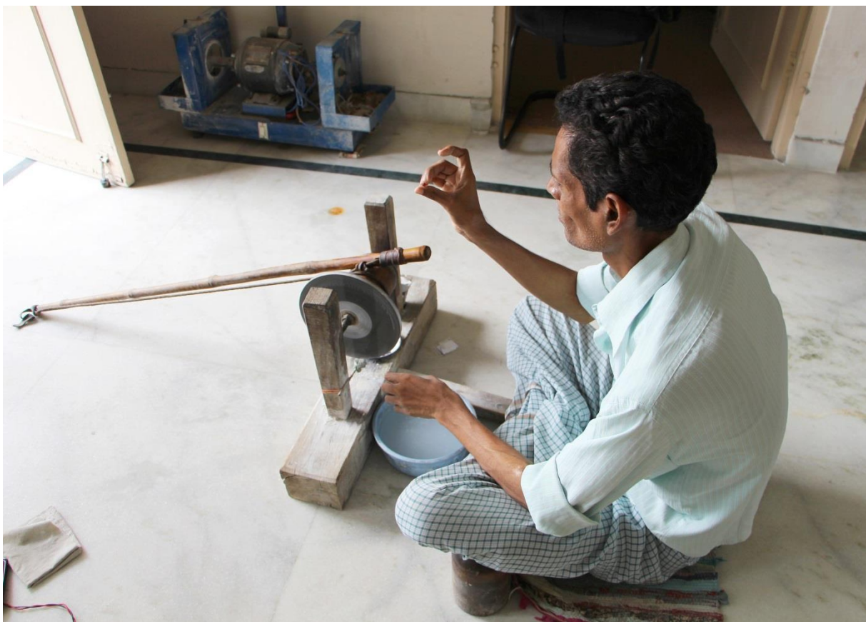
Fig. 7: Artisan processing a garnet using a jindrā in a workshop in Johari Bazaar, Jaipur. Photo: B. Larios, © Weltweites Zellwerk
